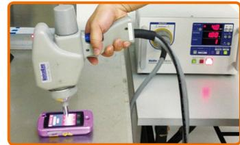
Static electricity tests
